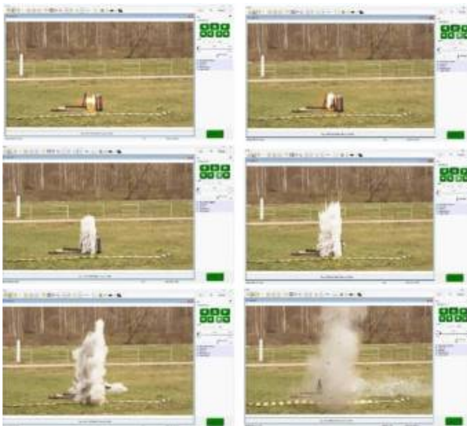
Figure 17. Frames with the functioning of liquid jet neutralisation device.
