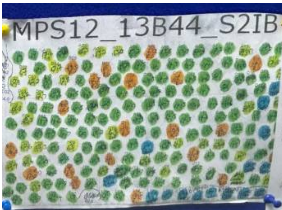
Figure 11. Example of a hot hole block (100 m x 60 m) where all holes have been charged (November 2024).
