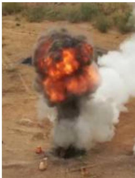
Figure 2. Spontaneous detonation of inhibited emulsion in lined hot hole.
