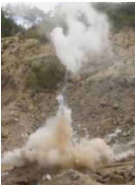
Figure 6. Apparatus with 4 chimney sections detonation.
