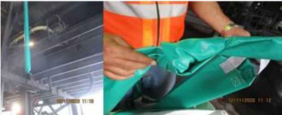
Figure 4. Images of PVC sleeve filled with water - strength tests, knot at bottom.
