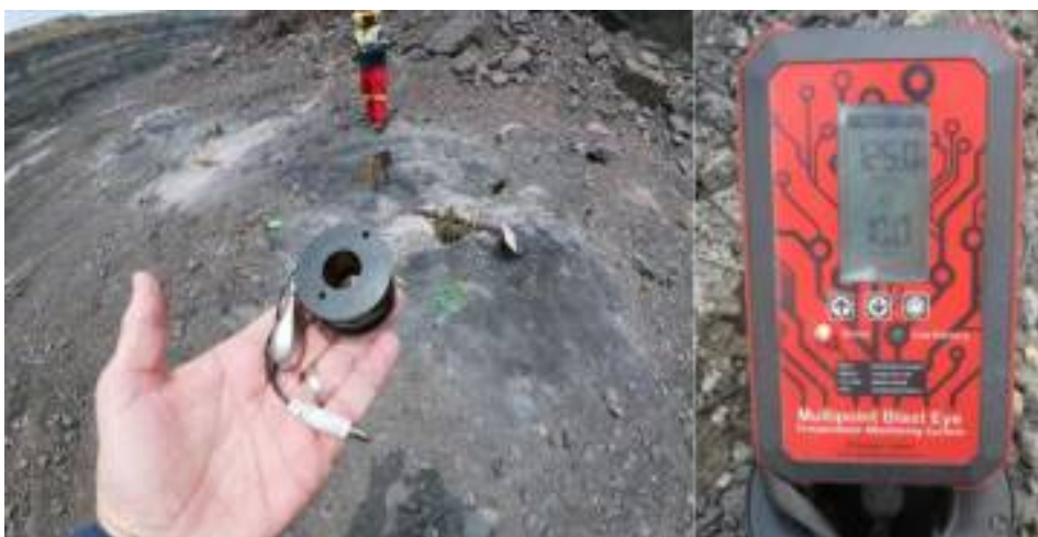
Figure 9. Multipoint Blast Eye cable and reader unit used on all sleeved holes above 80°C (Stenzel 2025).
