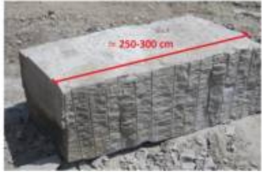
Figure 4. On the left side, the blasted rock block is shown resting on a debris bed, positioned after the initial detonation. This large block is then divided into vertical slices, which are further separated along pre-induced vertical split planes. Each of these slices is subsequently laid on another debris bed to facilitate further handling. On the right side, the process continues as each vertical slice is further subdivided into smaller blocks of the desired volume, typically ranging from 2 to 6 m 3 , which are then ready for transport to the processing plant for cutting and finishing operations (Cardu & Todaro 2024).
