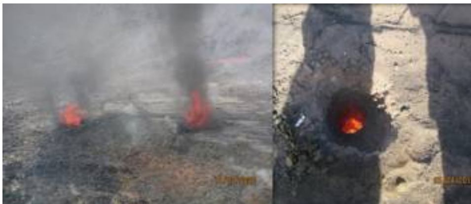
Figure 1. Fires in old underground workings (left & right). This burden must be blasted (G Stenzel 2019, 2020).
