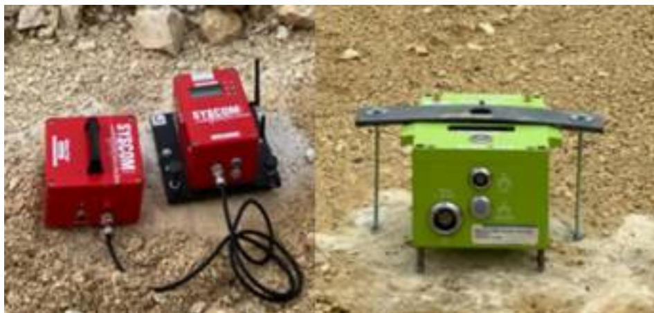
Figure 2. Seismographs used for this study: Menhir (left) and SYSCOM (right).
