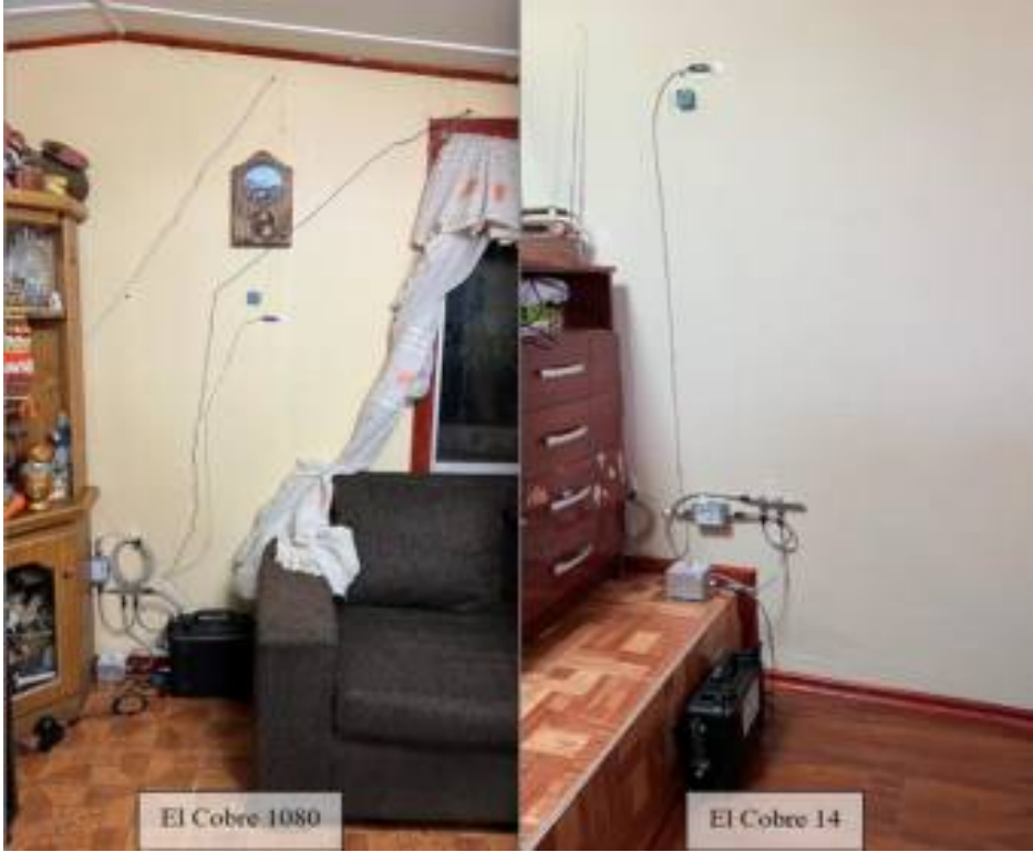
Figure 2. Instrumentation setup inside the monitored homes, including extensometers, triaxial geophones, and temperature and humidity sensors installed at El Cobre 1080 and El Cobre 14.
