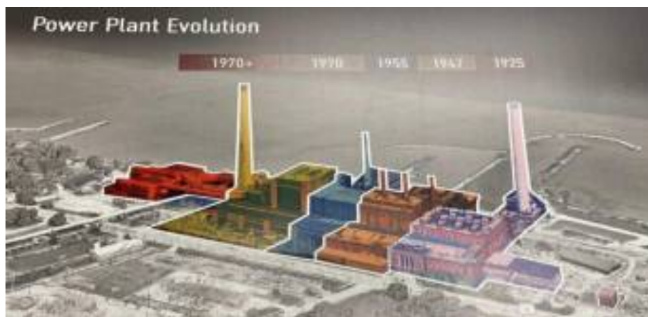
Figure 2. Construction sequencing for Avon Lake.
