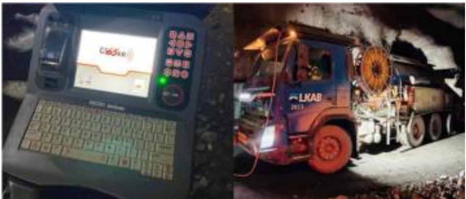
Figure 5(c & d). Instrumentation used for borehole filming: (c) RIDGID CS65xr digital monitor (left); (d) LKAB's charging truck (right).
