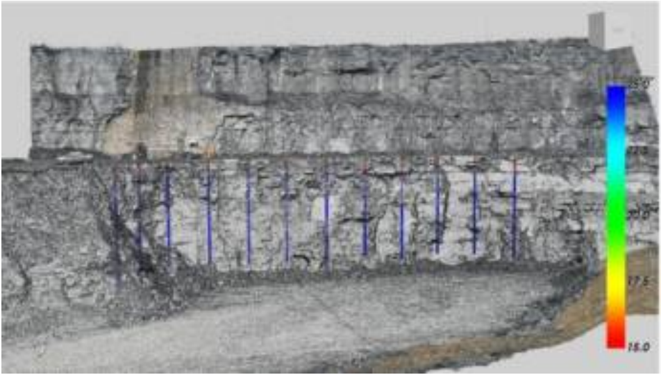
Figure 2. Interpretation of MWD results showing the estimated Young's elastic modulus.
