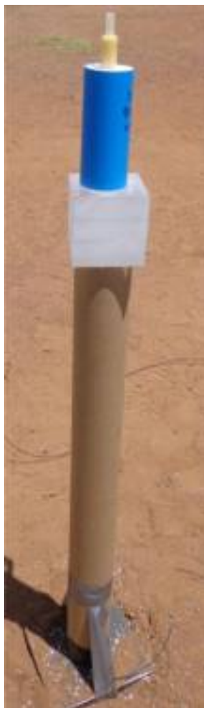
Figure 2. Large scale gap test setup (picture courtesy of Dr Henco Bezuidenhout).
