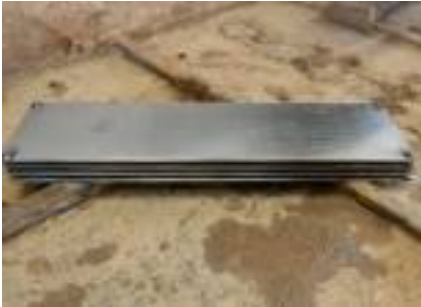
Figure 5. Four sheets of pure Nickel before shot with distance holders. The fifth sheet is absent to show the positioning of the distance sticks.
