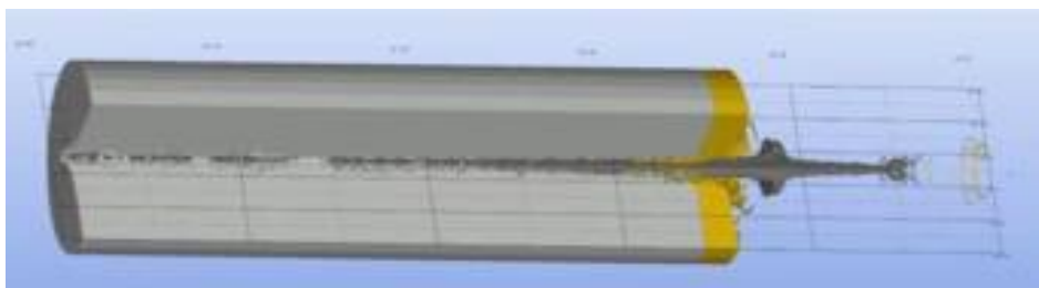
Figure 3. Shape charge detonation computer model.
