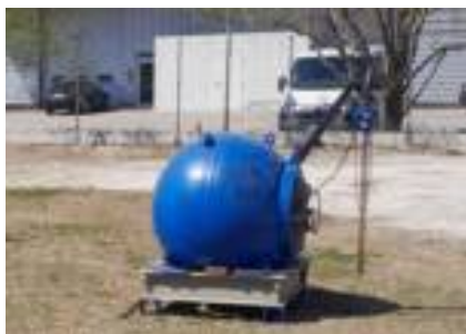
Figure 1. Explosive chamber prepared for test.
