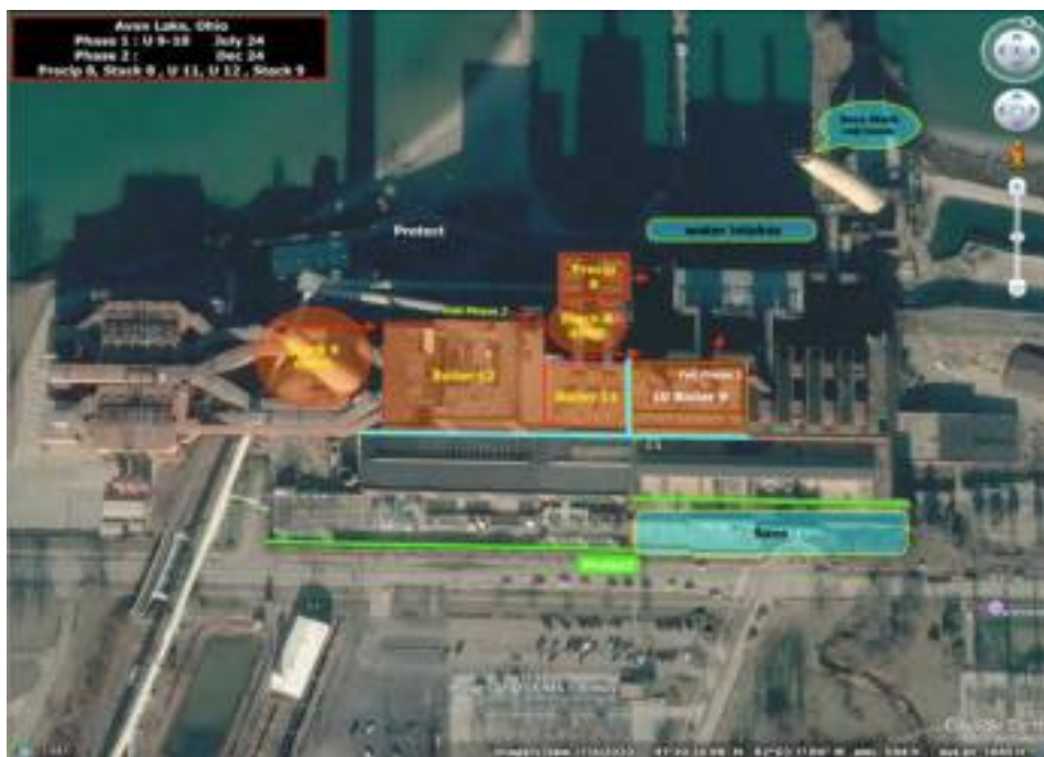
Figure 3. Avon Lake structure fall directions.
