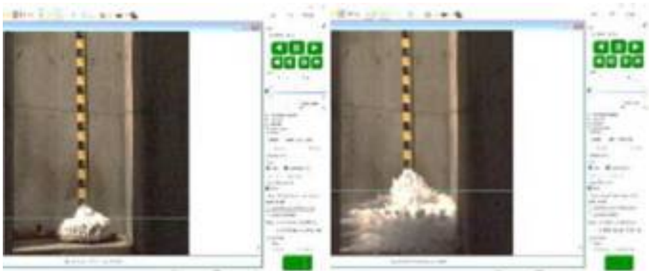
Figure 11. Liquid jet velocity of a) (left) 1080 m/s at 200 mm and b) (right) 560 m/s at 300 mm.
