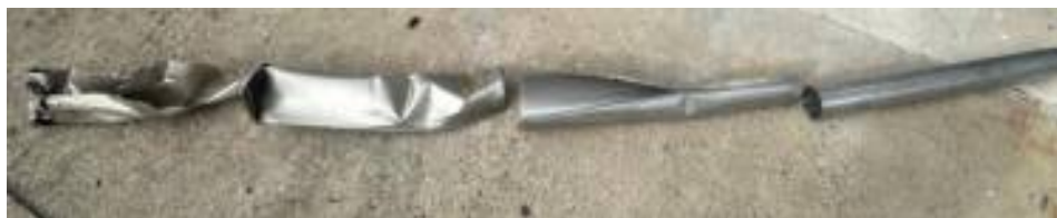
Figure 7. Recovered chimney sections show hydrogen detonation of hydrogen in chimney and it appears there is deformation from the shock of the ammonium nitrate detonating.
