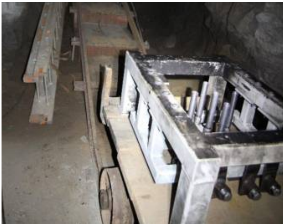
Figure 9. Sample holder for stability tests with passive gauges (material: lead) with rails for moving heavy samples in the lab itself (see also Figure 3).
