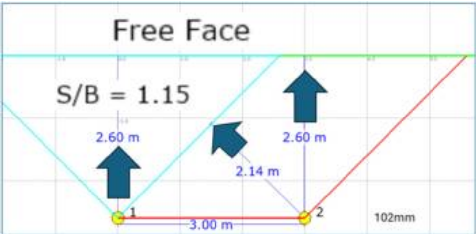
Figure 2. Plane section at the toe area of the first 2 blast holes in a SLC ring 2.6mB/3mS, blasting up to the free face.
