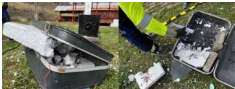
Figure 16. Destruction of the electrical circuit between the 'detonator' - mobile phone and explosive.
