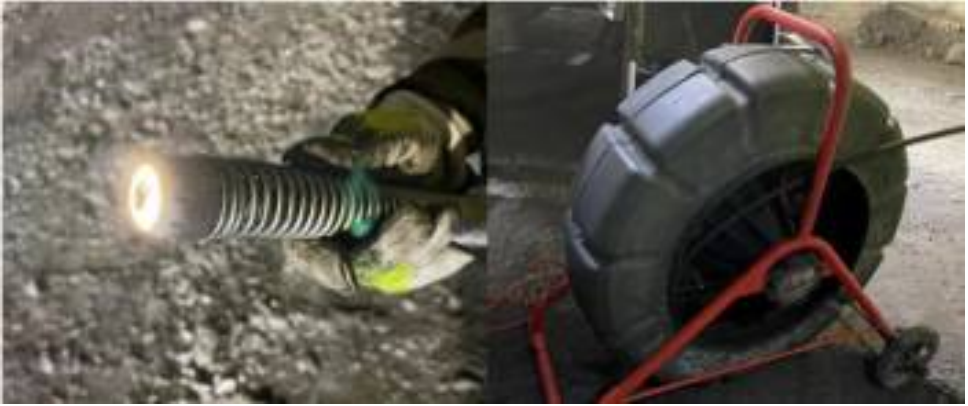
Figure 5(a & b). Instrumentation used for borehole filming: (a) RIDGID SeeSnake camera (left); (b) RIDGID standard reel with the 99 m long push cable (right).
