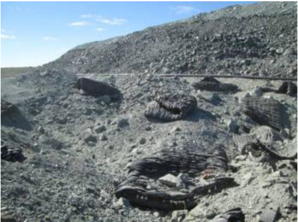
Figure 9. Flying blasting mats.
